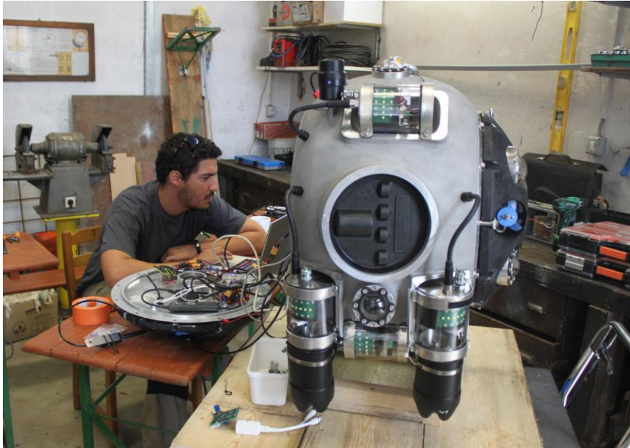
Figure 10. Troubleshooting of Vender Electronic Speed Controller (VESC).
