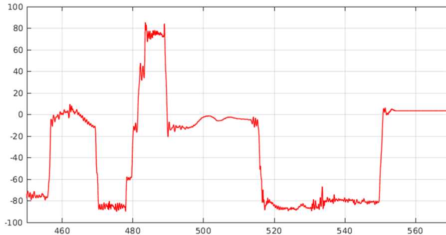
Figure 26. Pitch (deg) vs. time graph of nose down manoeuvre tests.
