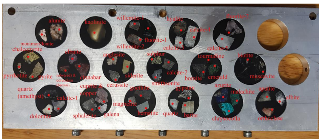
Figure 21. Reference sets of minerals prepared by the University of Miskolc, which were placed under water in the Idrija shaft in order to obtain reference spectra in real mine conditions.
