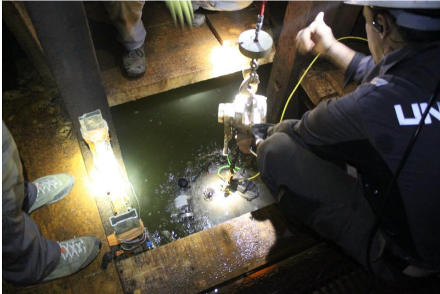
Figure 14. Launch of the UX-1a into Borba shaft.
